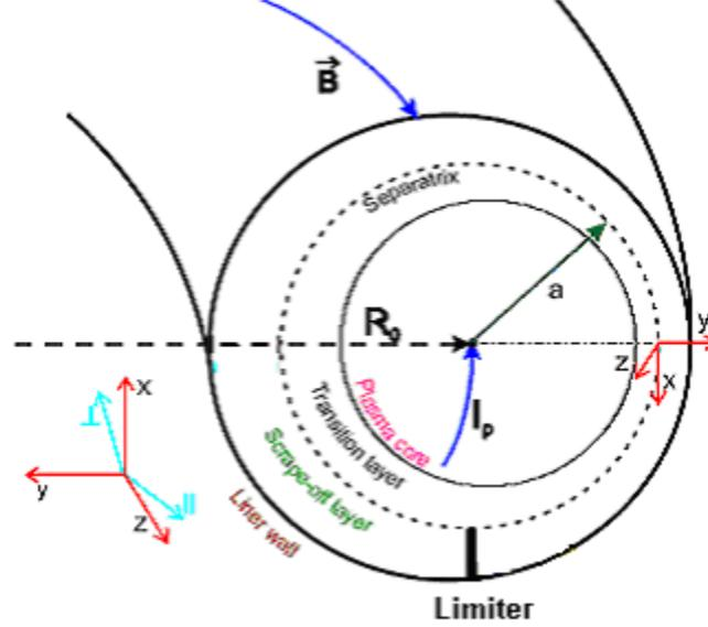
Fig. 3 Boundary layer geometry for tokamak plasma with toroidal limiter
