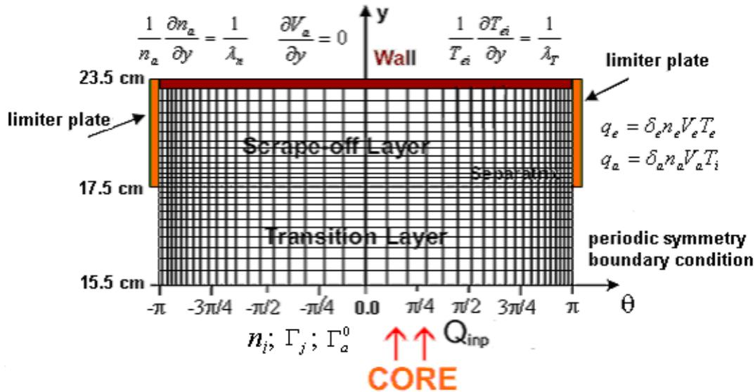
Fig. 5 Numerical mesh and boundary conditions
