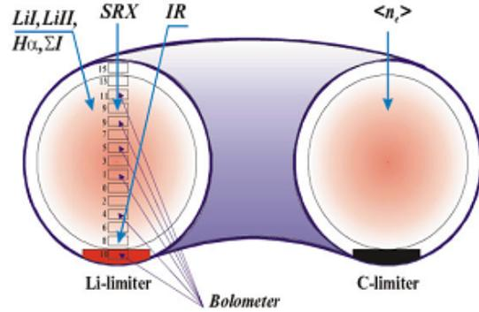
Fig. 1 Location of limiters and diagnostics in T-11M tokamak
