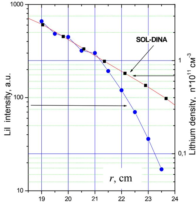
Fig. 11 Comparison between the experimental and simulated Lithium ion distributions in SOL
