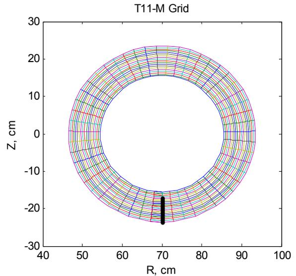
Fig. 4 Grid of transition layer and SOL area
