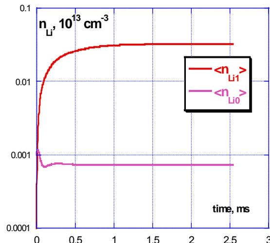
Fig. 14 Time traces of ions and neutral density of Lithium
