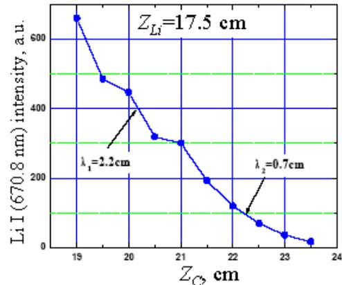
Fig. 2 Lithium flux radial distribution in the SOL plasma of T-11M [10]
