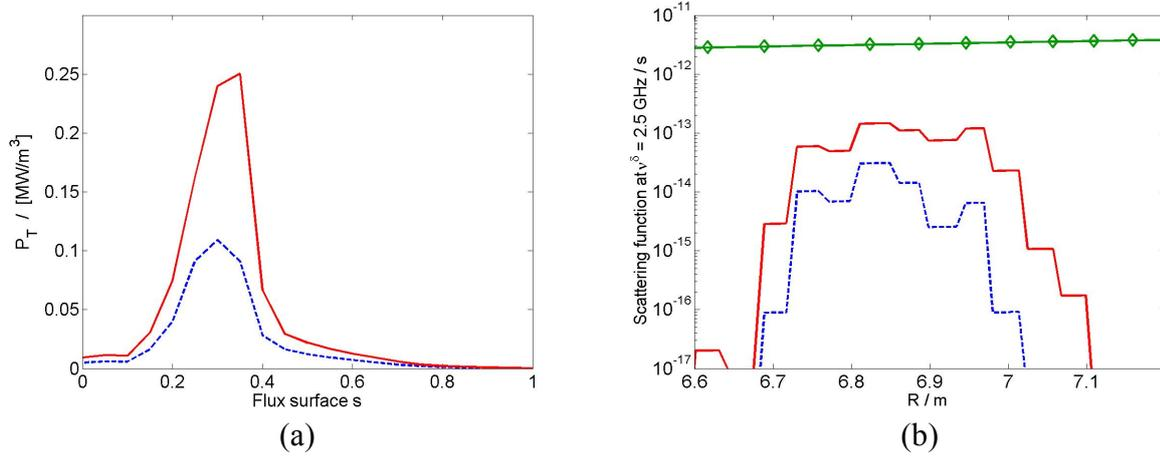
FIG. 3. Power deposition and scattering function profiles for pure second harmonic tritium heating; (a) Power deposition profile on tritons: — 40 MW, - - - 20 MW; (b) Scattering function at  $\nu^\delta = 2.5$  GHz for various scattering volumes with different R;  $\blacklozenge$ - alphas, — tritons at 40 MW, - - - tritons at 20 MW
