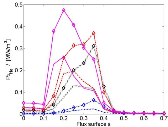
FIG. 5. Power deposition profiles on  $^3\text{He}$  for various  $^3\text{He}$  concentrations and heating powers; curves with symbols – 40 MW, curves without symbols – 20 MW; concentrations: — 4%, - - - 2%,  $\cdots$  1%, - · - 0.1%
