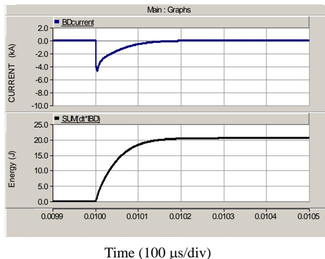
FIG. 5. Simulated waveforms of breakdown current and input energy into the accelerator.
