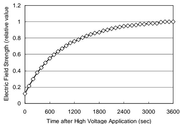
FIG. 4. Time variation of electric field strength in the insulation of transformers.
