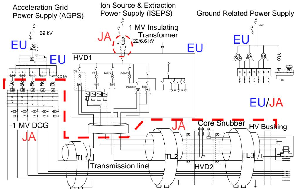
FIG. 1. ITER NBI Power supply system.
