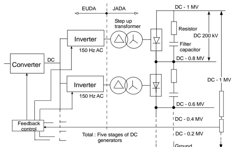
FIG. 2. -1 MV AGPS system and its control system.
