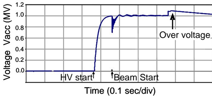
FIG. 3. Simulated waveform the AGPS output.
