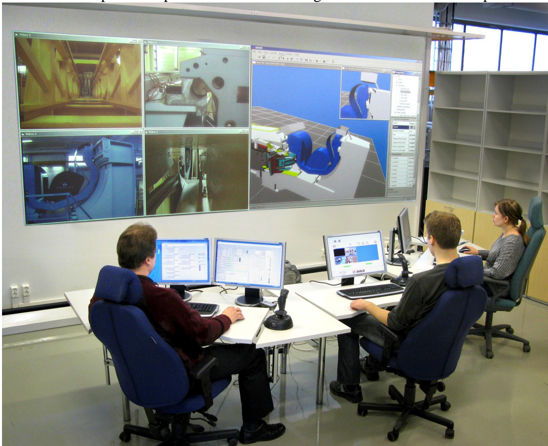
Figure 6. Operators in DTP2 control room use camera view and virtual model to control the divertor maintenance devices.
