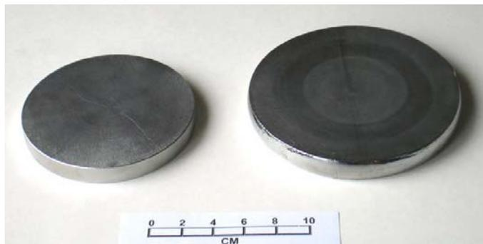
Figure 1. Large single crystal molybdenum mirror substrates
