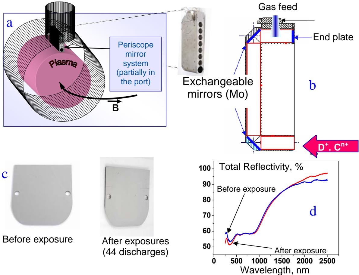
Figure 2. Details of the exposure of Periscope mirror system in TEXTOR: a) scheme of exposure; b) scheme of Periscope mirror system; c) photographs of first mirrors before and after exposure and d) evolution of the total reflectivity of the first mirrors before and after exposure, as measured at the center of the mirrors.
