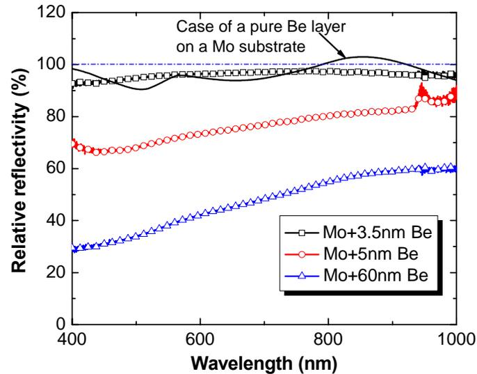
Figure 3. Relative reflectivity of Be deposits on molybdenum mirrors from [19]. The black line corresponds to the relative reflectivity of Be and Mo from [17] and corresponds to the reflectivity which should be measured if the mirror consisted of a perfectly smooth Be layer deposited on the polished substrate. The dashed line at 100% indicates the reference level corresponding to a non-exposed mirror.
