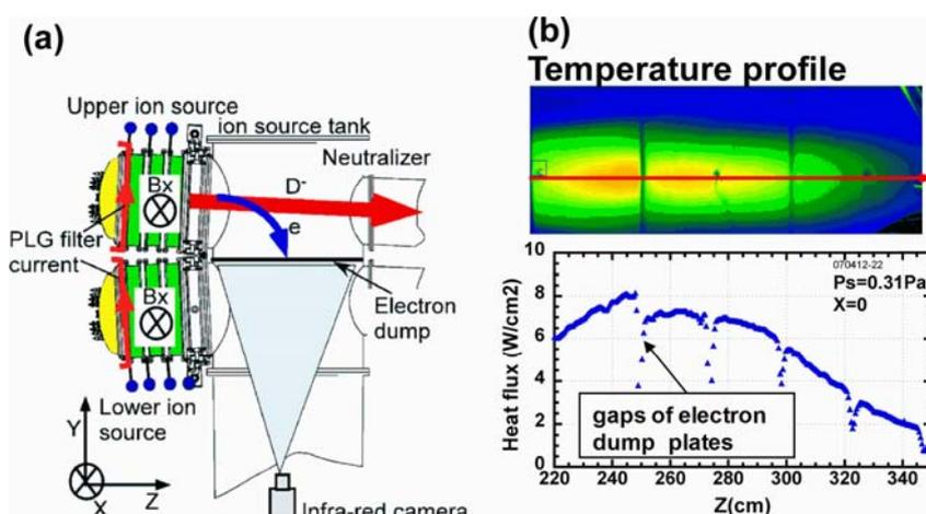
Figure 3 (a) Set up of electron deposition measurement, (b) temperature and heat flux profiles at the electron dump.
