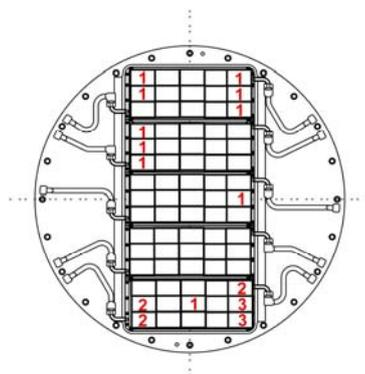
Figure 2 Breakdown location on the acceleration grid in the U ion source.
