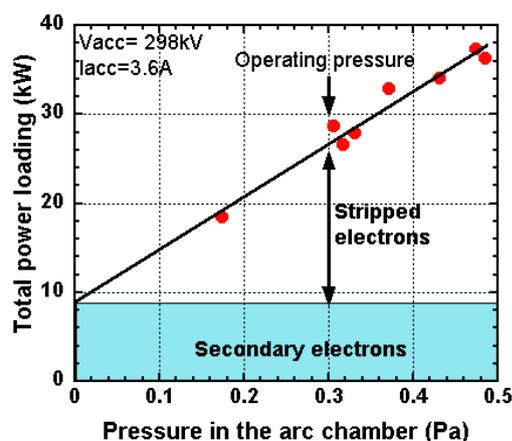
Figure 4 Total power loading as a function of the pressure in the ion source.
