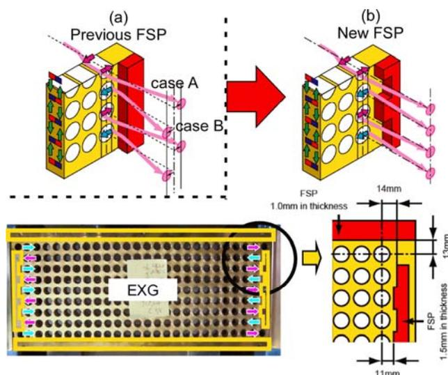
Figure 5 Previous (a) and new (b) field shaping plates.
