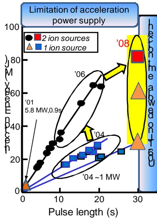
Figure 7 Progress of the long pulse injection of the  $D^0$  beams on JT-60U
