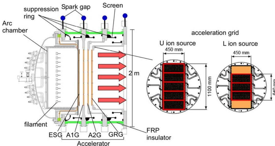
Figure 1 Schematic diagram of the JT-60 negative ion source
