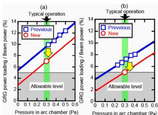
Figure 6 Power loadings of the grounded grids in the L (a) and U (b) ion sources.
