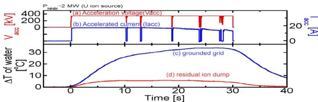
Figure 8 Time evolutions of acceleration voltage (a), accelerated current (b), water temperature rises of grounded grid (c) and residual ion dump(d).
