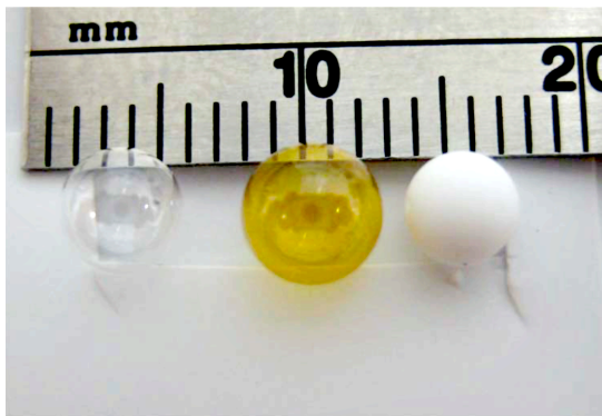
Fig. 5. Three shells: Left, a 4 mm diameter Poly alpha methyl styrene (PAMS) shell with a wall thickness of \sim 35 micron; Center, 5 mm diameter Glow Discharge Polymer (GDP) shell with wall thickness of \sim 20 micron (composition \sim \text{CH}_{1.2} ); Right, a 4 mm diameter Divinyl Benzene (DVB) foam shell with wall thickness of \sim 260 micron and open cell size of \sim 1 micron.
