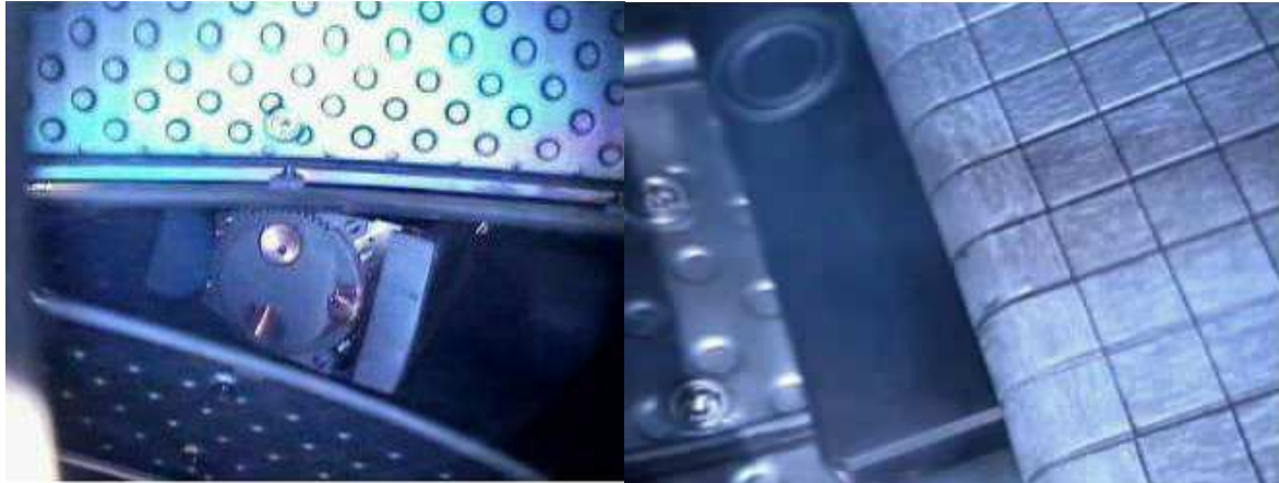
FIG. 5. Visual inspection of a Plasma diagnostics (under ultra high vacuum and at 120°C On the left: control of the shutter movement of an upper infrared endoscope On the right: close tracking of the bottom limiter surface and carbon tiles macroscopic analysis (the gap between the vision tool and carbon tile's limiter was kept at 10 cm)
