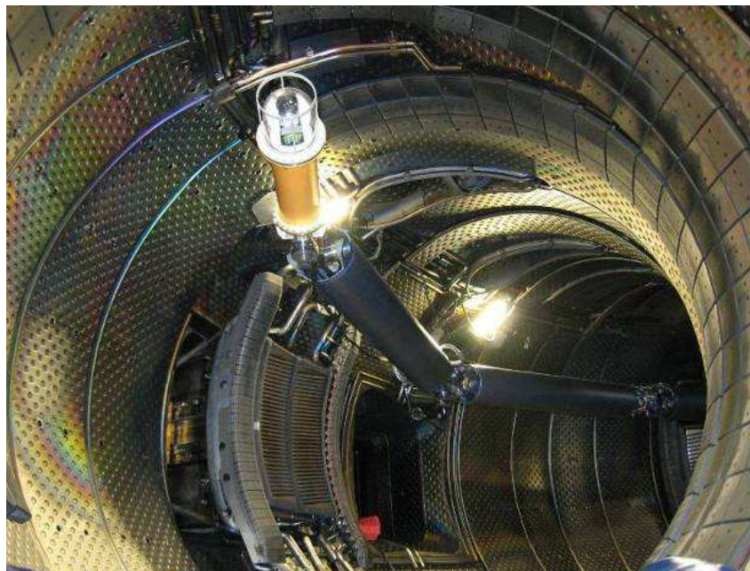
FIG. 4. On the left: AIA with the viewing system inside Tore Supra tokamak (atm. Pressure and 20°C).
