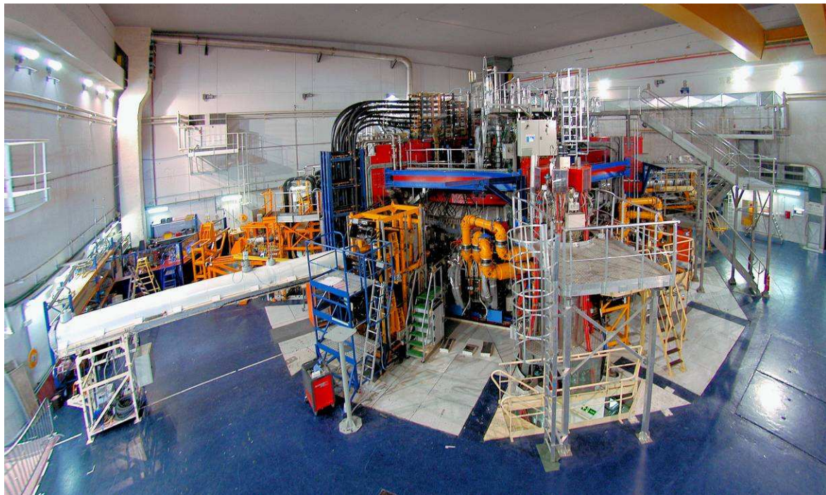
FIG. 3. The Housing of the AIA (white cask on the left) connected to the Tore Supra tokamak.
