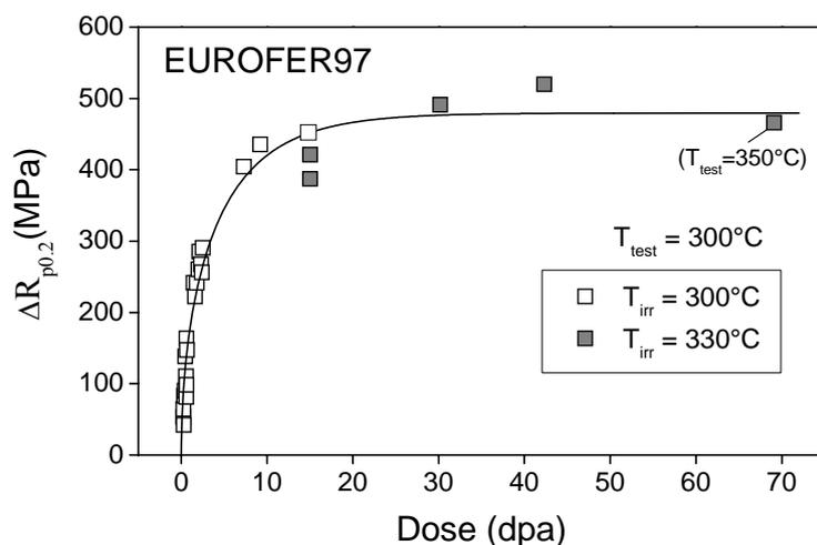
FIG. 2. Irradiation hardening vs. irradiation dose for  $T_{irr}=300$ - $330$  °C and  $T_{test}=300$  °C (exception: specimen from ARBOR 2 is tested at  $T_{test}=350$  °C) of EUROFER97. For comparative purposes the low dose data from [2,3] are also included. The line is a model description of the entire data set.
