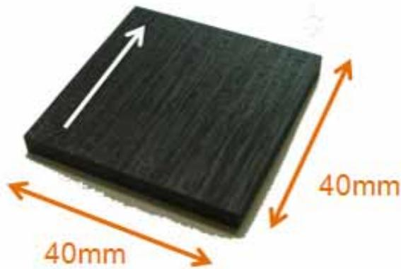
FIG. 3. Picture of the unidirectional NITE-SiC<sub>f</sub>/SiC composite prepared as a reference specimen.
