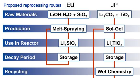
FIG.9. Fabrication flow of  $\text{Li}_2\text{TiO}_3$  and  $\text{Li}_4\text{SiO}_4$  pebbles.
