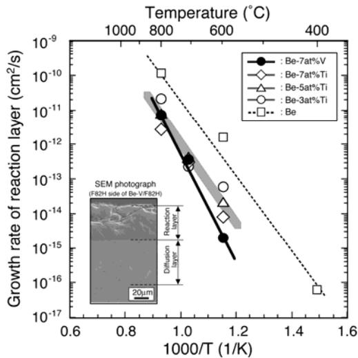
FIG.7. Growth rate of reaction layer of beryllium and beryllium-based intermetallic compounds on F82H as a function of the reciprocal temperature.
