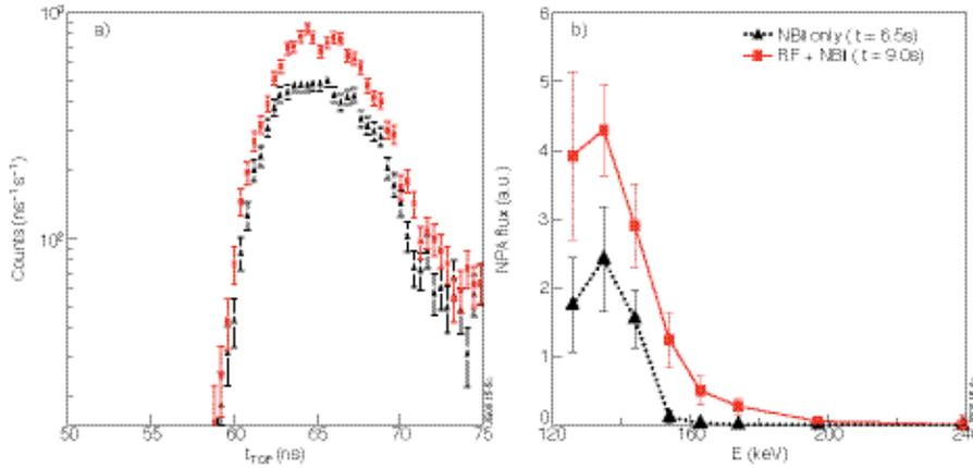
Figure 5: (a) Neutron counts from D-D reactions (~2.5MeV) as function of time-of-flight measured with the neutron spectrometer TOFOR in two phases of discharge #68288: (▲) NBI only and (■) combined ICRF+NBI; (b) Neutral particle fluxes (in a.u.) measured by the horizontal NPA system (KR2) as function of the fast D energy in two phases of discharge #68288: (▲) NBI only and (■) combined ICRF + NBI.
