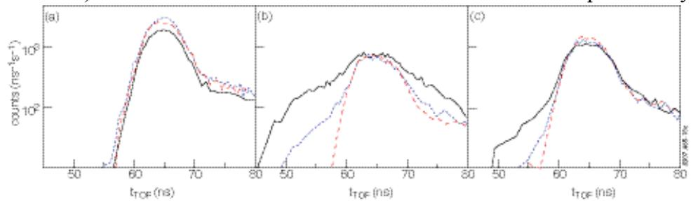
Fig. 6: Neutron time of flight spectra (number of counts as function of flight-time) from the TOFOR neutron spectrometer. Data are shown for JET pulse 69388 (a), pulse 69392 (b) and 69393 (c). For each pulse spectra are shown for three different subsequent time slices during the magnetic field flat top RF+NBI phase: short dashes for t=5-6s, long dashes for t = 6-7s, solid lines for t= 7-8s.
