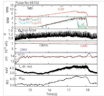
**Figure 3.** Example of a JET ELMy H-mode with up to 8MW coupled ICRF power at a ROG of 14 cm and D<sub>2</sub> gas injected from GIM 6, 9 and 10.
