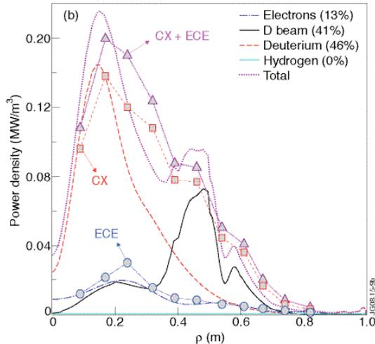
Fig. 4: Power absorption profiles obtained with the full-wave CYRANO code for the fundamental D heating scenario in JET using the particle distributions computed from the quasi-linear Fokker-Planck code BATCH to represent the NBI deuterons. The experimental power deposition profiles for the electrons and the bulk ions obtained by ‘break-in-slope’ analysis of the ECE (●) and CX (■) signals in discharge #68733 are also included.
