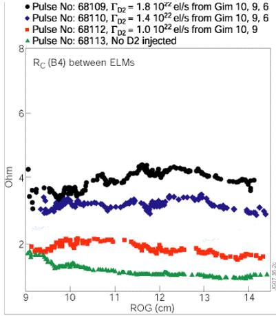
**Fig. 1.** Evolution of the coupling resistance of the B4 antenna strap as a function of ROG and for different levels of D<sub>2</sub> gas injected (using various combinations of GIMs)
