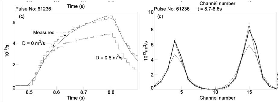
Fig.8. 14MeV neutron rate plot (left) comparing measured and calculated with  $D_{an}=0$  (dotted) and  $D_{an}=0.5\text{m}^2/\text{s}$  (dashed) for pulse 61236 (on-axis T) and 14MeV profile (right) comparing measured (solid) with  $D_{an}=0$  (dotted) and  $D_{an}=0.5\text{m}^2/\text{s}$  (dashed) simulation). The profiles are integrated over 100ms, the error bars from a single profile (integrated over 10ms).
