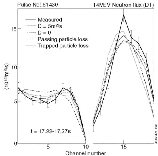
Fig.9. Profiles of 14MeV neutron emission with different forms of anomalous fast ion losses #61430.
