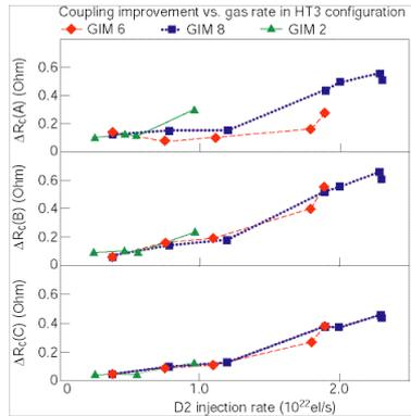
**Figure 2.** Effect of D<sub>2</sub> gas injection from GIM 6 and GIM 8 on the baseline coupling (i.e. coupling between ELMs) of JET A2 antennae A, B and C.
