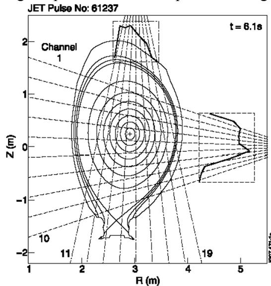
Fig. 7. Lines of sight of the neutron camera on JET with channel numbers and a typical profile shape for off-axis NBI heating.
