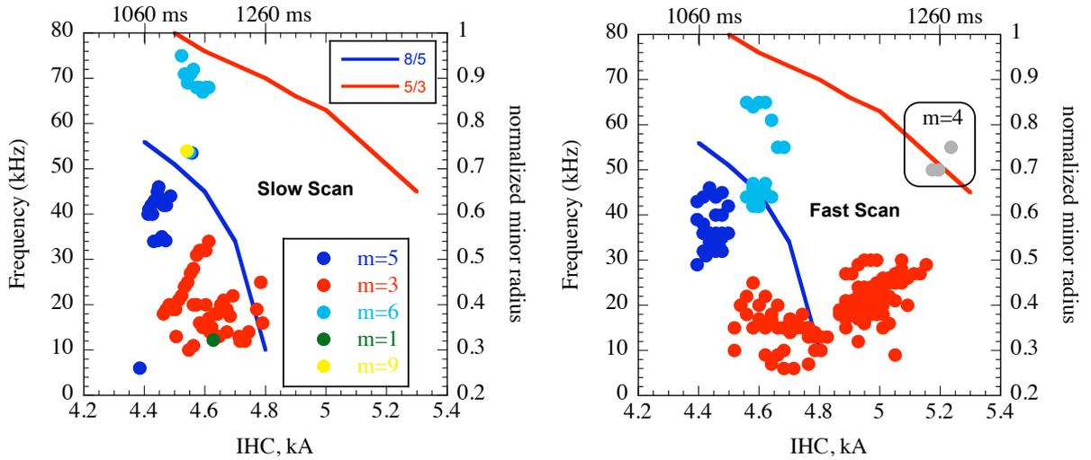
FIG. 4. Frequencies and poloidal mode numbers as a function of the currents in the helical conductor in slow (left) and fast (right) scan discharges. The corresponding times of the discharges are shown above.
