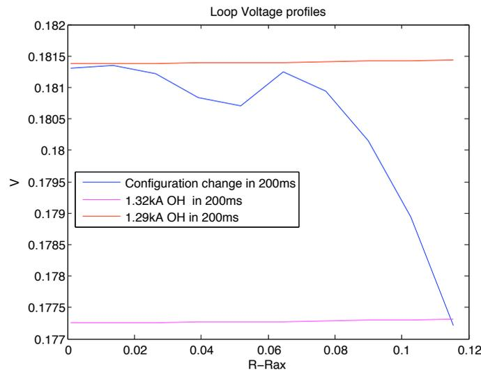
FIG. 2. Calculated radial profiles of loop voltage due to a linear change of magnetic configuration with HC varying from 4.4 to 4.8 kA in 200 ms; and two values of loop voltage due to linear ramps in the OH coils.
