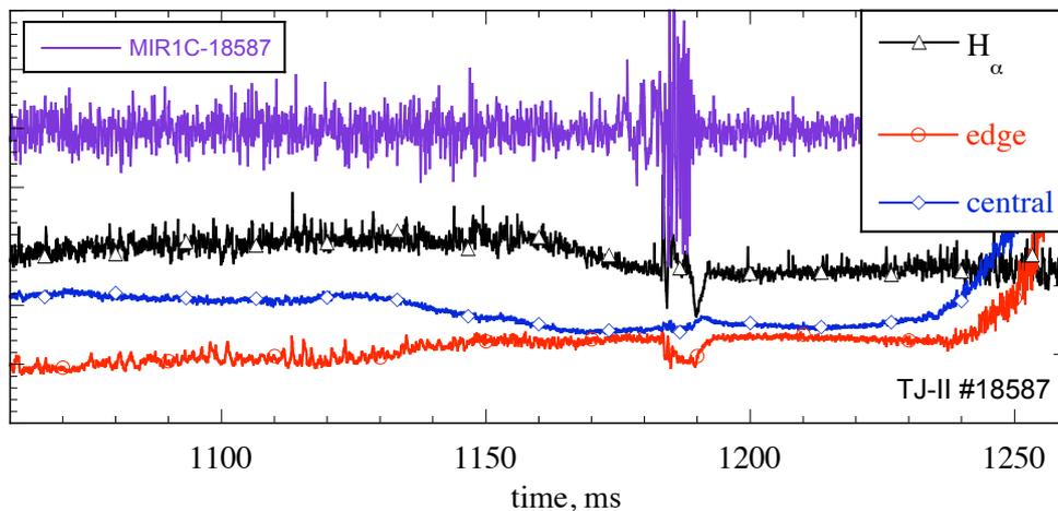
FIG. 7. From top to bottom: time traces (arbitrary units) of Mirnov coil,  $H_\alpha$  monitor, and edge and central bolometer chords for TJ-II discharge #18587.
