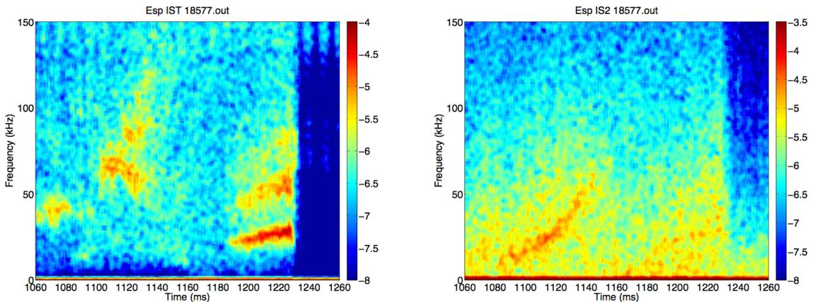
FIG. 5. Spectrograms of the signals of a magnetic probe ( $\rho \approx 1.05$ , left) and the saturation current of a Langmuir probe ( $\rho \approx 0.95$ , right) for the fast scan discharge TJ-II #18577. The discharge is terminated at  $t \approx 1230$  ms due to ECH density cut-off limit.
