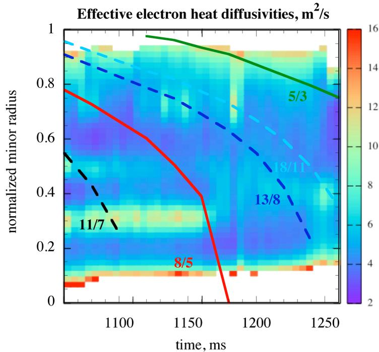
FIG. 6. Contour map of the effective electron thermal diffusivity ( $\sim 1/L_{Te}$ ) during a fast configuration change experiment. Lowest order magnetic resonances of the calculated vacuum rotational transform are traced with lines. White areas correspond to out of range data.
