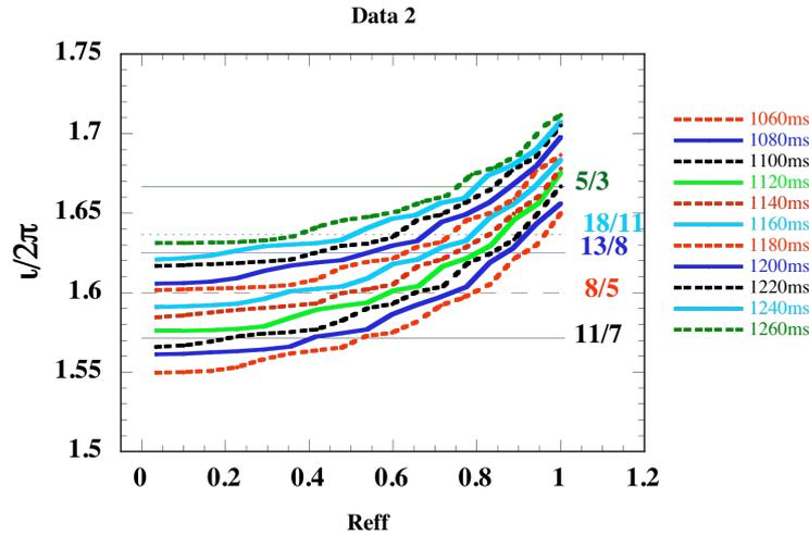
FIG. 1. Rotational transform profiles for several vacuum magnetic configurations obtained by changing (mainly) the current in the helical conductor. Several magnetic resonances move inwards in radius as the edge  $t$  increases. In a dynamic configuration experiment, these vacuum configurations coincide with discharge times like those labeled on the right.
