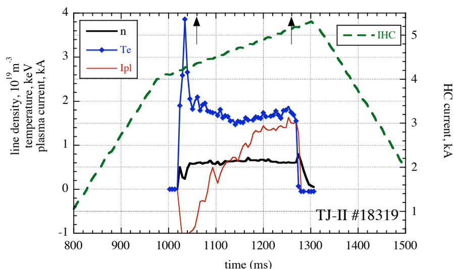
FIG. 3. Time traces of line density (thick line), core electron temperature (diamonds), net plasma current (thin line) and current in the helical conductor (dashes) for TJ-II discharge #18319. The arrows indicate times at which the vacuum configuration is coincident with configurations of the TJ-II flexibility diagram.
