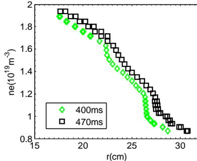
FIG. 8. The density profile by microwave reflectometry in different time in shot 8264. The particle transport barrier position is about  $r=26 \text{ cm}$ . Line average density is about  $2.2 \times 10^{19} \text{ m}^{-3}$ , the power of the ECRH heating is about 200 kW.
