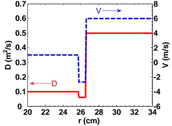
FIG. 5. Diffusivity  $D$  (solid), convective velocity  $V$  (dash) for the simulation of shot #7593.
