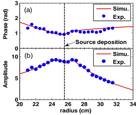
FIG. 4. Shot #7593. Phase (a), amplitude (b) of the 1st harmonic of the Fourier transform of the modulated density. Comparison between experiment (circle) and simulation (solid).
