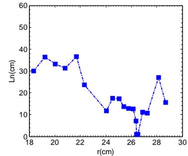
FIG. 9. The density gradient length of shot 8264 at  $t=400 \text{ ms}$ . The minimum value is smaller than value in figure 3. It shows that the particle transport barrier in ECRH is stranger than that in pure Ohmic discharge.
