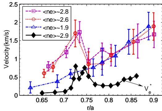
FIG. 6. Radial profile of the perpendicular turbulence rotation velocity with pITB ( $\circ, \square$ ) without pITB ( $\Delta$ ) measured by Doppler reflectometry. Radial profile of the electron diamagnetic drift velocity  $V_e^*$ .
