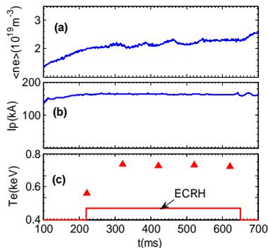
FIG. 7. The evolution of the parameters in ECRH heating in shot 8264: (a) the line average density by HCN, (b) the plasma current and (c) the electron temperature by Thomson scattering.
