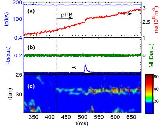
FIG. 2. Shot #7557. (a) Temporal evolution of the plasma current  $I_p$  (kA), the central line averaged density  $n_l$  ( $10^{19}m^{-3}$ ). (b) Temporal evolution of the Mirnov coil signal and  $H_a$  signal. (c) 2-D image of the density gradient.
