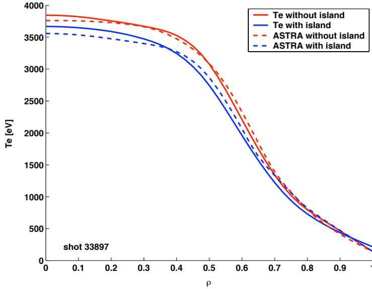
**FIGURE 5.** Comparison of electron temperature experimental profiles (lines) and ASTRA modeling results (dots) for pre-MHD, top-performance state (red), and island saturation phase (blue)
