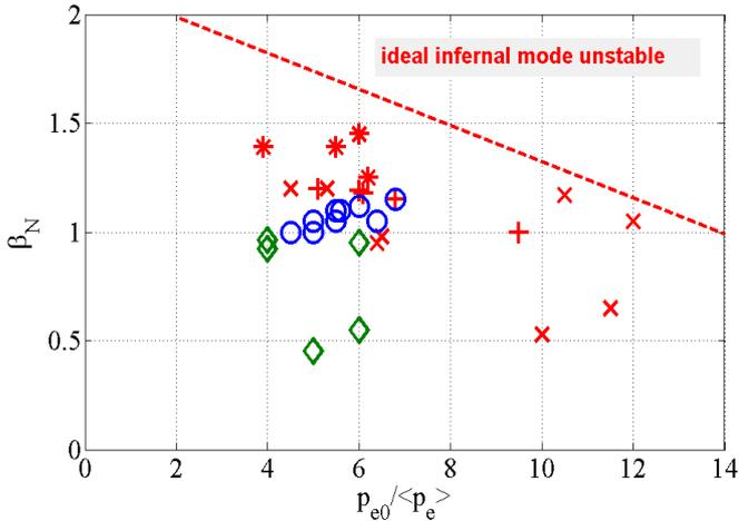
**FIGURE 2.** Measured  $\beta_N$  versus the pressure peaking factor,  $p_e(0)/\langle p_e \rangle$  for discharges featuring global plasma oscillations caused by ideal MHD (red marks; “\*” are for shots close to a major disruption, “X” are for shots with periodic crash-like global oscillations, “+” are for small fast crashes with amplitude  $\Delta T_e/\langle T_e \rangle < 20\%$ ), resistive MHD (blue circles) and discharges with MHD activity but without global oscillations (green diamonds).
