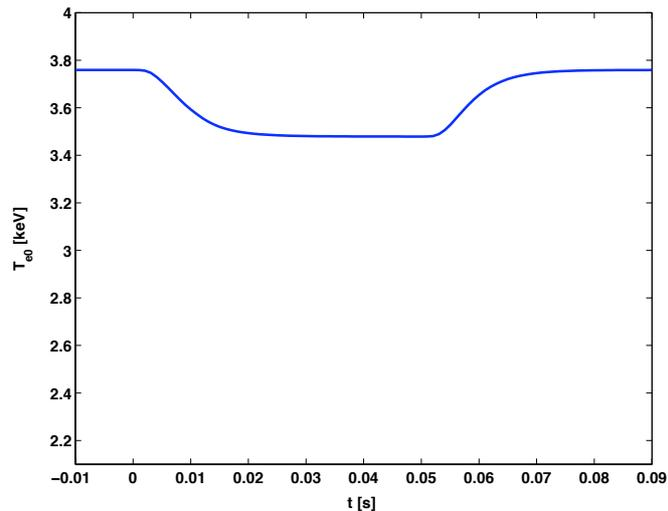
**FIGURE 7.** ASTRA central electron temperature time evolution during the modeled appearance of the island. The new stationary state is reached in 20 ms, with a central drop of almost 300 eV.
