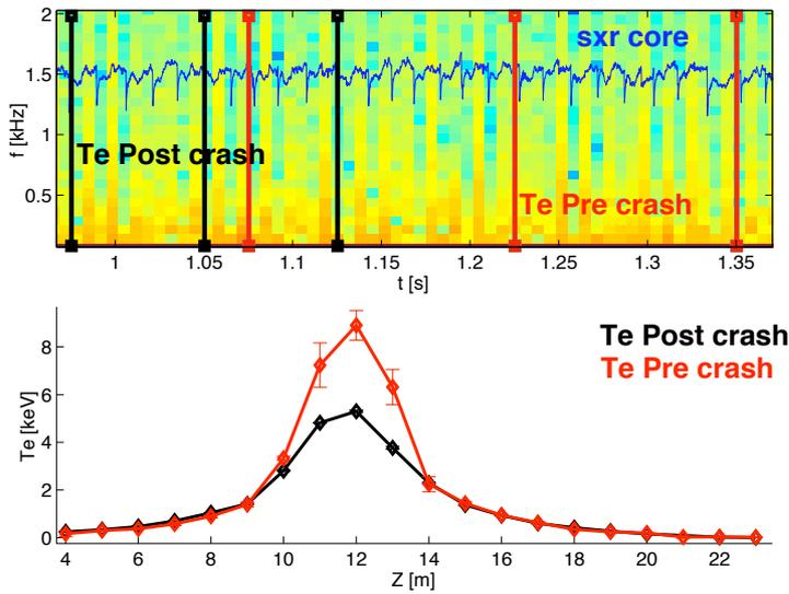
**FIGURE 4.** Shot 24696 Thomson Scattering (TS) data. The top plot show sSXR spectrogram and SXR core raw trace (blue) evidencing the periodic crashes. The red lines shows TS profiles of pre-crash states, whereas the black one are taken during post-crashes states. The bottom plot reports the profiles, indicating the loss of electron temperature.
