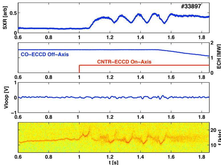
**FIGURE 1.** (a) Evolution of the main plasma parameters in fully non-inductive discharge #33897. The top trace is core SXR, which indicates the barrier formation ( $t=1.08$ s) and the onset of the global oscillations ( $t=1.2$  s). The combination of co and counter-ECCD is displayed in the second plot. The  $v_{loop}$  (bottom trace) shows the plasma is fully non inductive and the bottom trace shows the spectrogram of Mirnov probe signal.
