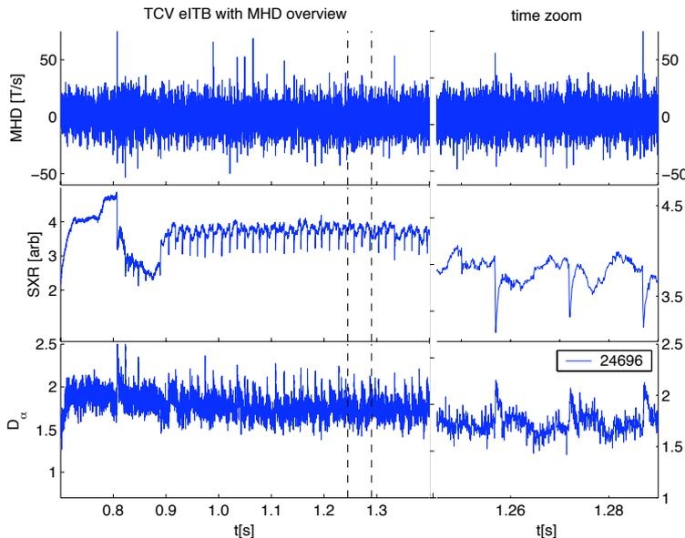
**FIGURE 3.** Shot 24696 overview. The top trace shows the Mirnov probe signal, indicating with the spikes the ideal activity at the crashes. The middle trace shows SXR core emission, with the periodic crashes after the eITB formation. The bottom trace shows  $D_\alpha$  emission. On the right box, the zoom of the indicated time window is reported.
