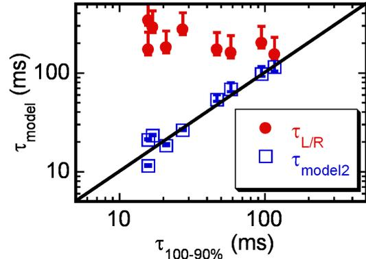
FIG.9. The comparison of the experimental value and the model prediction value of current decay time in initial phase of current quench.
