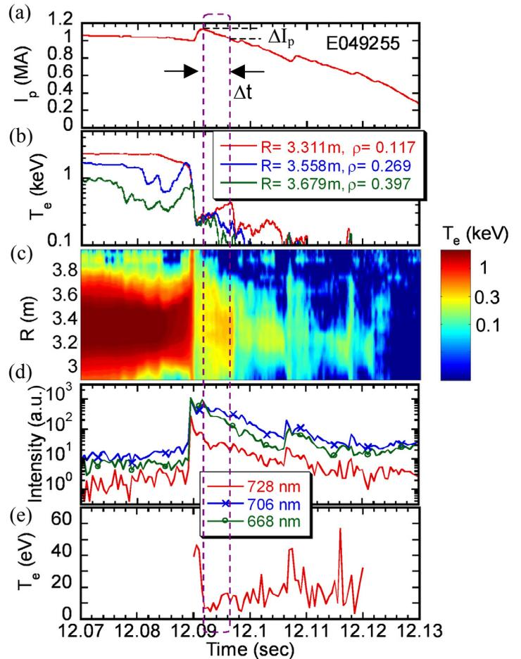
FIG. 2. The evaluation of (a) plasma current  $I_p$  and (b) electron temperature  $T_e$  measured by ECE diagnostic system, (c) major radial profile of  $T_e$ , (d) He I emission intensity and (e) electron temperature by using HeI emission Intensity ratios method.
