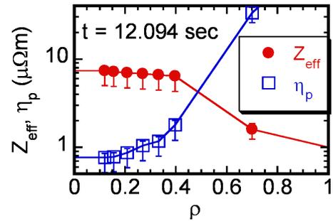
FIG. 5. Profile of plasma effective charge and resistivity at  $t = 12.094$  sec. The effective charge is calculated using the assumption of D : Ne = 9 : 1, 7 : 3 and 1 : 1.
