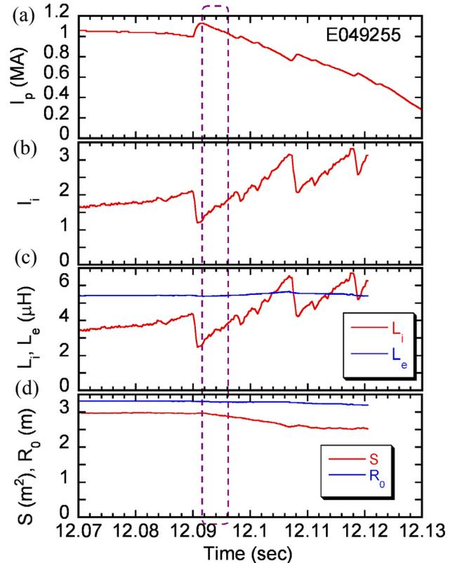
FIG. 7. The evolution of (a) plasma current, (b) plasma internal and inductance, (c) plasma internal and external inductance and (d) plasma cross-section and major radius evaluated by CCS method.
