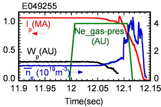
FIG. 1. The typical waveform of radiation induced disruption in JT-60U.
