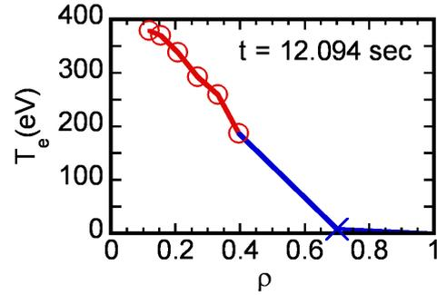
FIG. 4. Profile of electron temperature measured by ECE systems and He I spectroscopy at  $t = 12.094$  sec.
