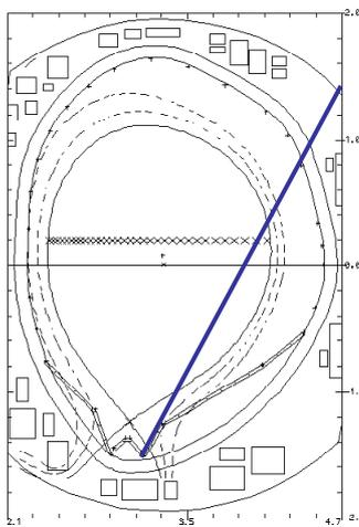
FIG. 3. Poloidal cross-section view of JT-60U plasma. Blue line means the line of sight for HeI spectroscopy.
