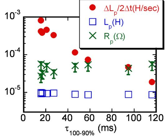
FIG. 8. The plasma resistance  $R_p$ , the plasma inductance  $L_p$  and the time change rate of the plasma inductance as a function of current decay time.
