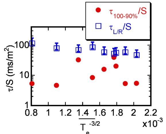
FIG. 6. The area-normalized current decay time as a function the area-averaged  $T_e^{-3/2}$
