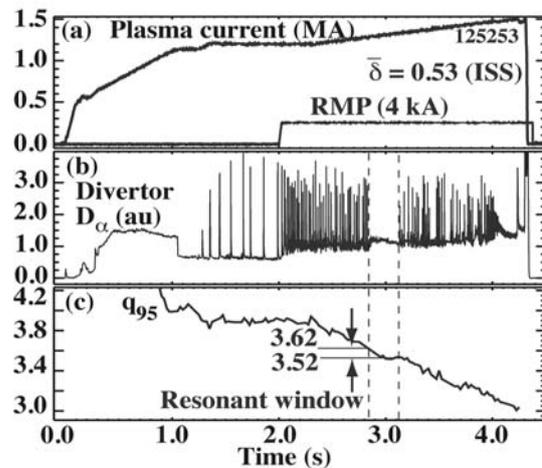
FIG. 2. An example of sharp  $q_{95}$  ELM suppression window in an ISS plasma with (a) an upward  $I_p$  ramp and 4 kA  $n=3$  RMP I-coil pulse producing (b) a quiescent interval in the lower divertor  $D_\alpha$  as (c)  $q_{95}$  passes through the region bounded by 3.62 and 3.52 during the downward ramp.
