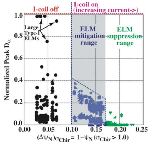
FIG. 5. The normalized peak in a divertor  $D_\alpha$  signal is well correlated with the width of the stochastic boundary layer when parameterized by the width of the region between the separatrix  $\psi_N = 1$  and the point in  $\psi_N$  where the Chirikov parameter crosses unity.
