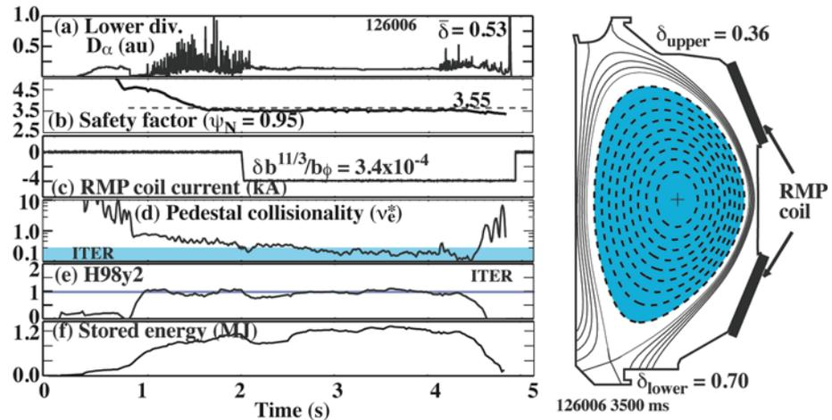
FIG. 1. Example of full ELM suppression in a low collisionality, high average triangularity DIII-D ISS plasma (discharge 126006). The plasma shape (right) at  $t = 3500$  ms is shown along with the location of the RMP coil (i.e., the DIII-D I-coil). On the left: (a) a typical lower divertor  $D_\alpha$  signal is shown along with (b) the evolution of  $q_{95}$ , (c) the RMP coil current, (d) the pedestal collisionality, (e) the H-factor and (f) the stored energy.
