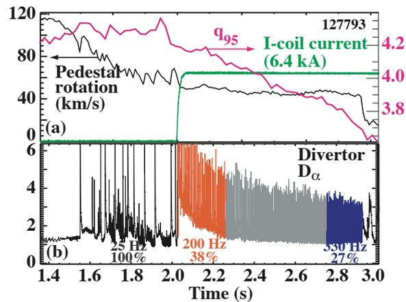
FIG. 4. Example of ELM mitigation in an ISS plasma where (a)  $q_{95}$  is ramped from 4.2 to 3.6 and the carbon VI toroidal rotation remains relatively constant (until a core MHD mode is destabilized a 2.9 s) during an  $n=3$  RMP pulse. Here, the (b) lower divertor  $D_\alpha$  signal that ELMs have a monotonically decreasing amplitude and increasing frequency during the RMP pulse compared to the Type-I ELM before the RMP pulse.
