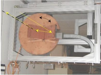
*FIG.7: Retro-reflector in the beam duct.*
