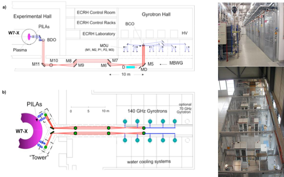
FIG. 1. The ECRH-plant for W7-X: Left: sketch of the gyrotron and transmission line arrangement in the ECRH-building, cross section (a) and top view (b). Right: Modular arrangement of Gyrotron and cooling units (top). HV-installation at ground-floor (bottom).
