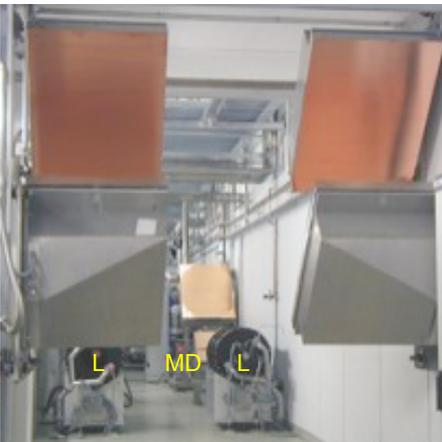
*FIG. 3. The W7-X quasi-optical transmission system. Top: Single beam section with BMO (M1,M2), short-pulse calorimeter (C), polarizers (P1,P2), microwave absorbers (AB1) and feeder mirror (M3) mounted on a common base frame. The beam path is indicated. Bottom: Section of the Multi-Beam-Waveguide, both cw-loads (L) are seen in the background.*
