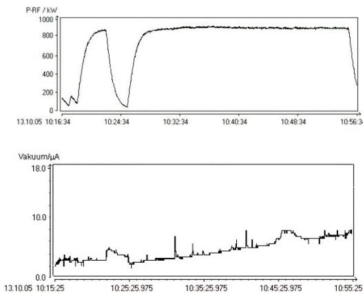
FIG. 6. TED SNo.1: RF-power (top) and gyrotron vacuum (GIP-current)(bottom) as a function of time (h.min.sec).
