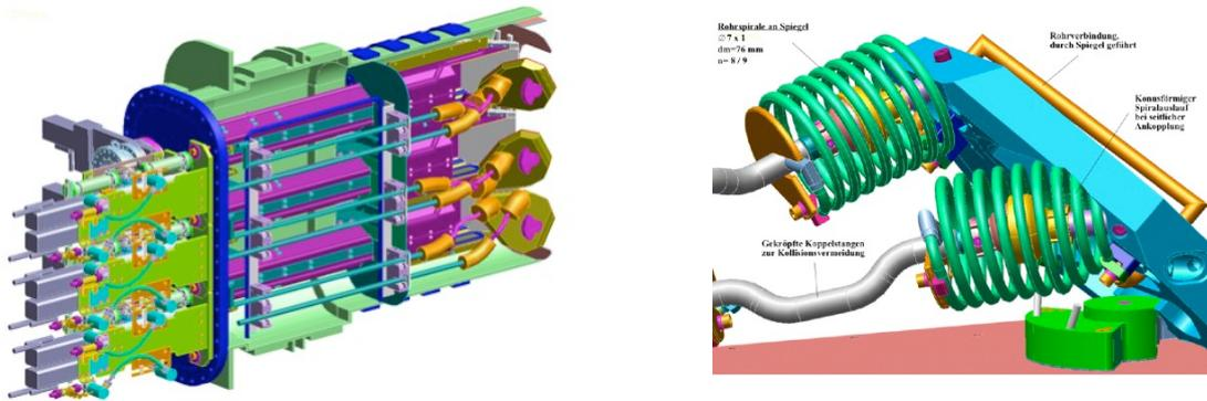
FIG. 4: Left: Front steering plug-in launcher. Right: Detail of the movable front mirror with driving rods and cooling spirals.
