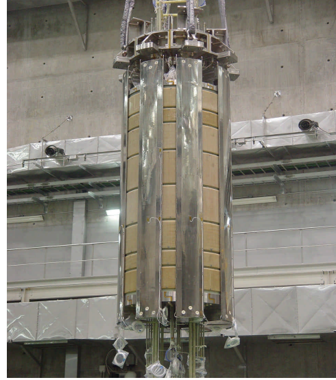
FIG. 13 CS coil after sub-assembly completion
