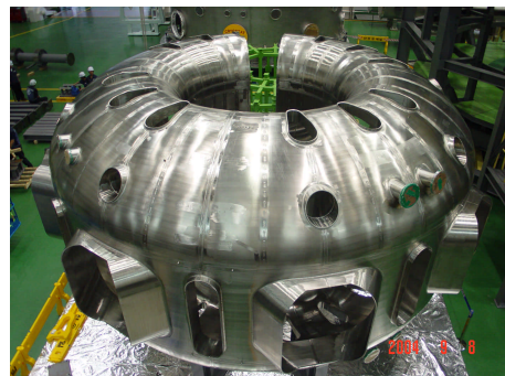
FIG. 6 337.5° sector of VV after site welding
