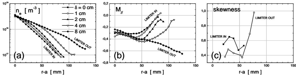
Fig. 6. (a) Radial density profiles measured on top of the torus by the Mach probe for five values of outboard clearance, (b) the corresponding profiles of parallel Mach number, and (c) the skewness of the probability distribution function of ion saturation current flowing to the probe from the low field side.
