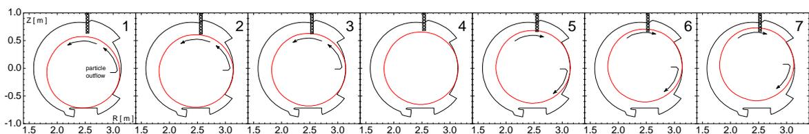
Fig. 3. Magnetic measurement of last closed flux surface as the plasma strike point is displaced upward along the outboard modular limiters. The arrows indicate the direction of flow past the Mach probe assuming that most of the SOL source is concentrated near the outboard midplane.
